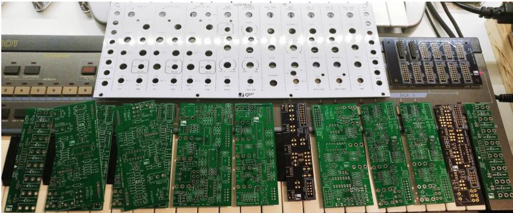
The ideal build plan starts with the patch board followed by the INPUT and OUTPUT boards. With those built and connected to the patch board various external inputs and outputs can be connected to test the other modules.
